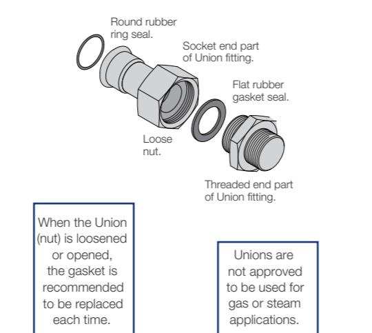
When the Union (nut) is loosened or opened, the gasket is recommended to be replaced each time.
