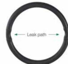
ConfitPRESS inox press-fit benefits from patented 'leak-before-press' O-ring technology which indicates if a joint has not been pressed. The O-ring contains two in-built water pathways that in the unpressed condition allows water to pass through and create a noticeable leak when the system is tested at low pressure (0.1 to 6.0 bar). Any unpressed joints can be pressed without draining down.
