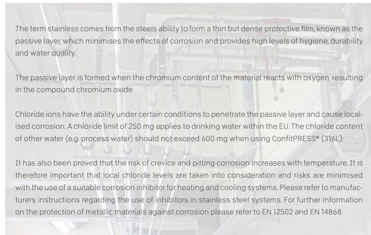
The term stainless comes from the steels ability to form a thin but dense protective film, known as the passive layer, which minimises the effects of corrosion and provides high levels of hygiene, durability and water quality.
