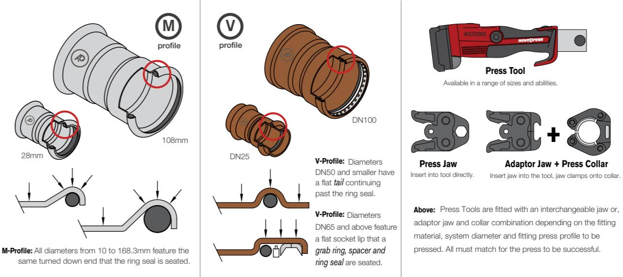
Since the original M-Profile was invented by Larsson, other profiles have been developed based on his design. Although appearing to be similar, each profile performs with different strength, deformation and ability characteristics.
