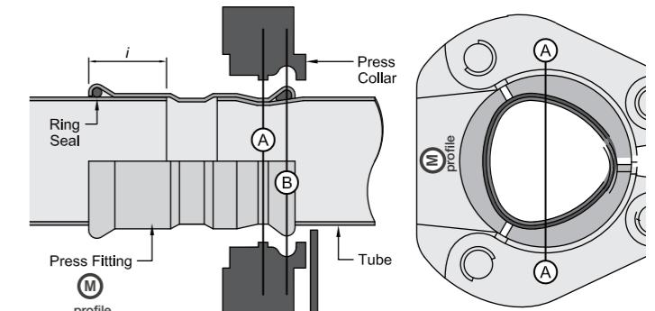
Above: Lemon shape section profile - Before pressing (fitting left), after pressing (fitting right) & Section A through pressed join
